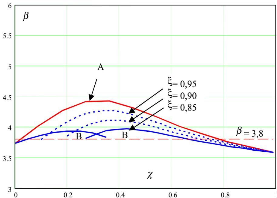
Figure 2.6: Variation of reliability index  $\beta$  with  $\chi$  for EN 1990 combination rules A ( $\gamma_R = 1,15$ ,  $\gamma_G = 1,35$ ,  $\gamma_Q = 1,5$ ) and B ( $\gamma_R = 1,15$ ,  $\gamma_G = 1,35$ ,  $\gamma_Q = 1,5$ ,  $\xi = 0,85, 0,90, 0,95$ ).  $k = 0$  (One variable action)
