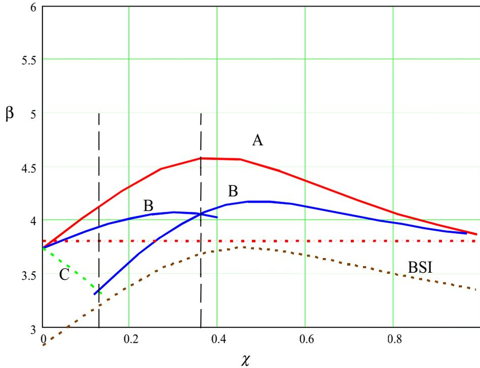
**Figure 2.5. Variation of reliability index  $\beta$  with  $\chi$  for the EN combination rules A, B and C, ( $\gamma_R = 1,15$ ,  $\gamma_G = 1,35$ ,  $\gamma_Q = 1,5$ ,  $\gamma_W = 1,5$ ,  $\psi_W = 0,5$ ), and the BSI rules ( $\gamma_R = 1,10$ ,  $\gamma_G = 1,2$ ,  $\gamma_Q = 1,2$ ,  $\gamma_W = 1,2$ ) for  $k = 0,25$  (two variable actions). (N.B.  $\chi = (Q_k + W_k)/(G_k + Q_k + W_k)$ ,  $k = W_k/Q_k$ )**
