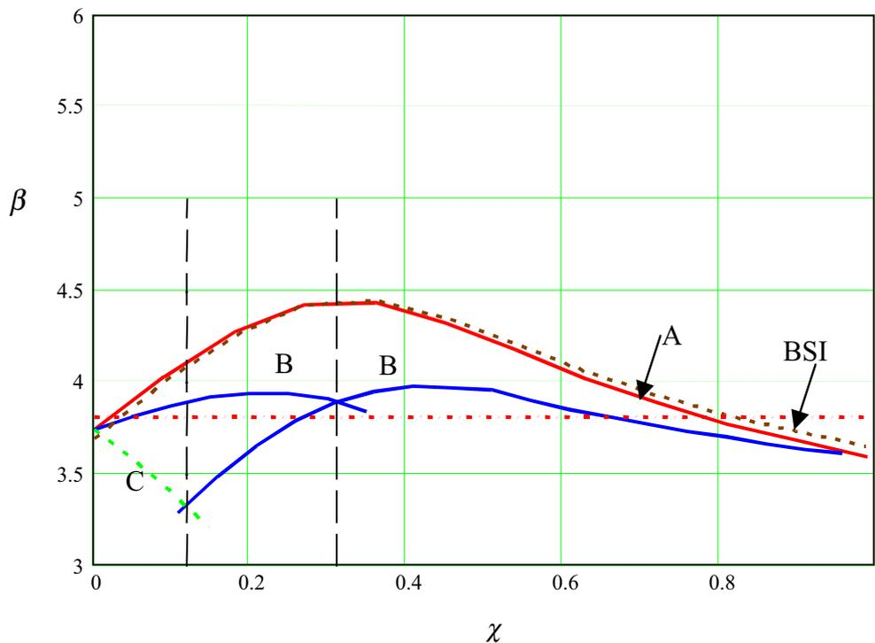
**Figure 2.4: Variation of reliability index  $\beta$  with  $\chi$  for EN 1990 combination rules A, B and C, ( $\gamma_R = 1,15$ ,  $\gamma_G = 1,35$ ,  $\gamma_Q = 1,5$ ), and BSI rules ( $\gamma_R = 1,10$ ,  $\gamma_G = 1,4$ ,  $\gamma_Q = 1,6$ ),  $k = 0$  (i.e. one variable action). (N.B.  $\chi = (Q_k + W_k)/(G_k + Q_k + W_k)$ ,  $k = W_k/Q_k$ )**
