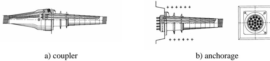
Figure 2: Coupling and anchorage devices
