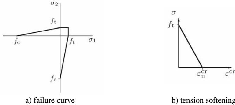
Figure 4: Concrete behaviour in tension
