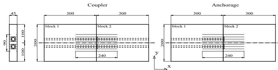
Figure 1: Model geometry
