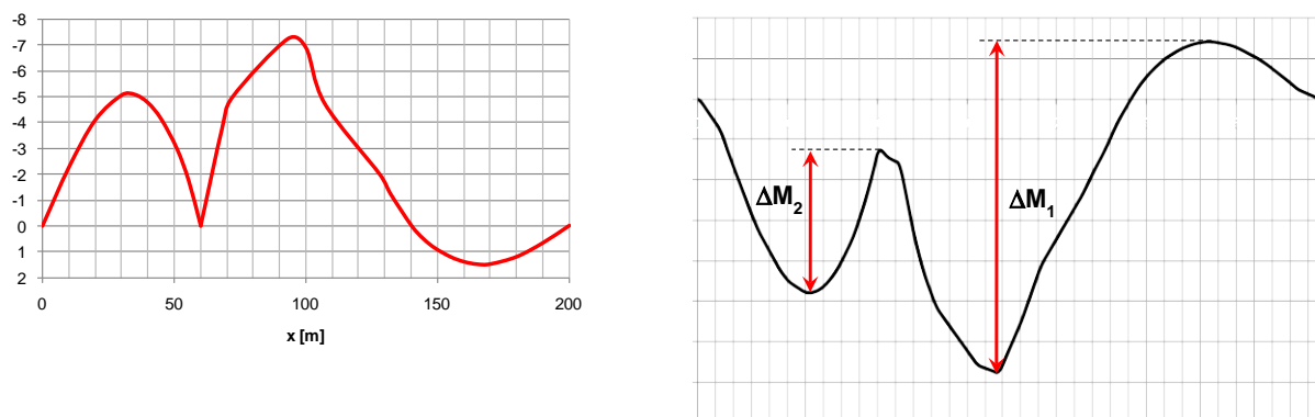
Fig. 3.22 Influence line and stress history induced by LM3 (cross section x=60 m, \eta=1 )
